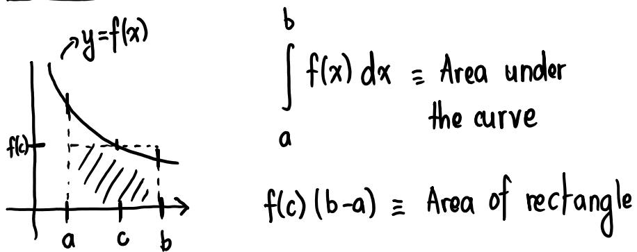
The MVT for integral states that for a positive function  $f$ , there exist a number  $c$  s.t. the rectangle w/ base  $[a,b]$  and height  $f(c)$  has the same area as the region under  $f$  betn  $a$  &  $b$ .  $\square$
